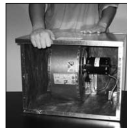
3. Rotate access panel 90°.
