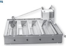
tight closure for exhaust units. Others are self-acting dampers that open and close automatically with the start/stop of the fan. There are low velocity standard duty and high velocity heavy duty styles. Dampers have aluminum, felted edges with interconnecting rods that prevent blade chatter or 'over-opening'. Damper frames are rugged, galvanized steel roll formed channels and are provided with a knock-out to permit the passage of electrical conduit.
